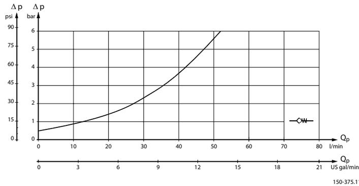
The check valve in the LS line of OSPC LS and OSPD LS dynamic steering units also protects the driver against steering wheel jerks. The check valve prevents oil from flowing backwards into the LS line to the priority valve when steering against a high pressure on the cylinder side.
