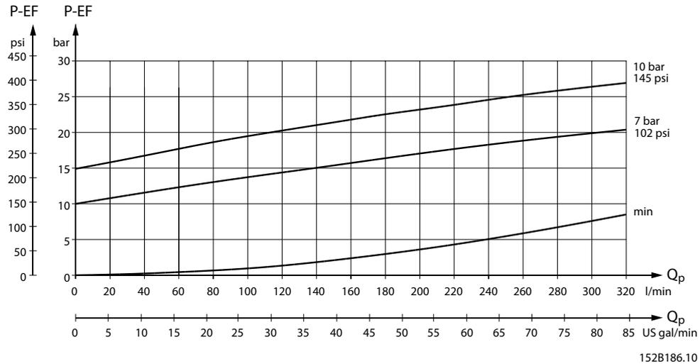
OLS 160 and OLS 320, pilot pressure relief valve (P - T, Qp) characteristics
