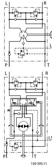
**OSPC LS: Steering unit load sensing with integrated valve functions for flange on priority valve OLSA**
