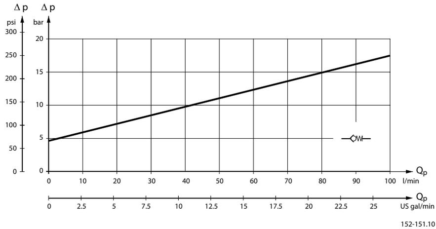
The curve below shows pressure drop for backpressure valve with by-pass.
