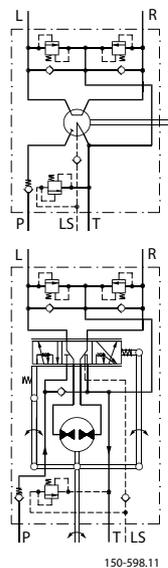
**OSPF LS : Steering unit full drain load sensing dynamic and with integrated valve functions**
