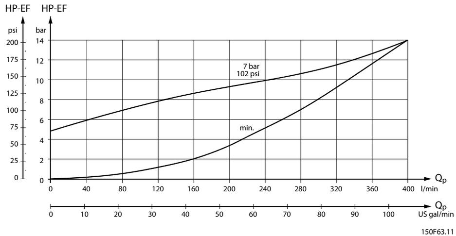
**OSQ pilot pressure relief valve (HP - HT, Qp) characteristic**
