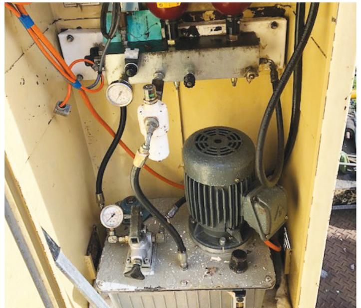
Hydraulics approximately 20 plus years ago. Given the age of the system, the technician stripped down the unit and thoroughly serviced and tested the system, hydraulically and electrically, restoring the brake unit to good working order for automatic function.
