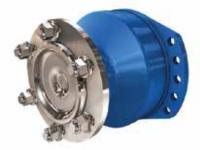
Poclain Hydraulics has become a world leader in hydrostatic transmissions based on their high performance direct drive cam-lobe radial-piston motors. These motors provide high efficiency and very low noise emission. Their motors offer a displacement range from 172cc up to 30,000cc and are also equipped with high radial and axial load capability bearing support, single or dual displacement, with or without brake.
